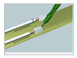
Use an operating tool or simply "twist and pull" to remove solid conductors.
