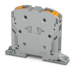
High-current terminal block, nom. voltage: 1000 V, nominal current: 232 A, connection method: Power-Turn connection, 1 level, cross section: 25 mm² - 95 mm², mounting type: direct screw connection, color: gray
