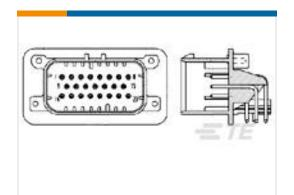
TE Part # 776280-1 8POS,PIN DIA 1.3,HDR ASSY,90DEG, COD 1
