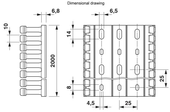
Base perforation according to DIN EN 50085
