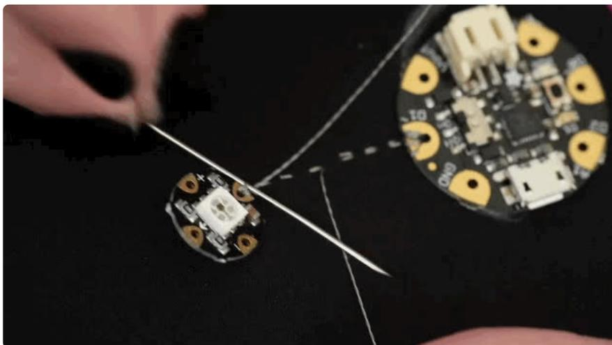
Make sure that each arrow points away from the microcontroller in a line. Stitch around the input pad tightly, even knotting the thread here to form an extra sturdy connection.
