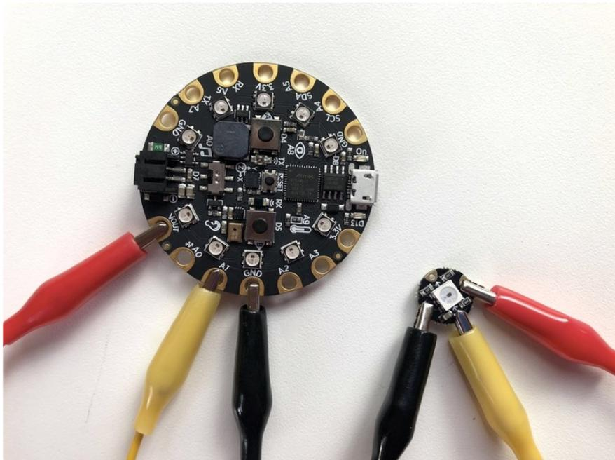
Hook up three alligator clips to your Circuit Playground Express as shown: one to **VOUT**, one to **A1**, and one to **GND**. I used a red wire for power and a black wire for ground for clarity, but it doesn't matter what color you use.
