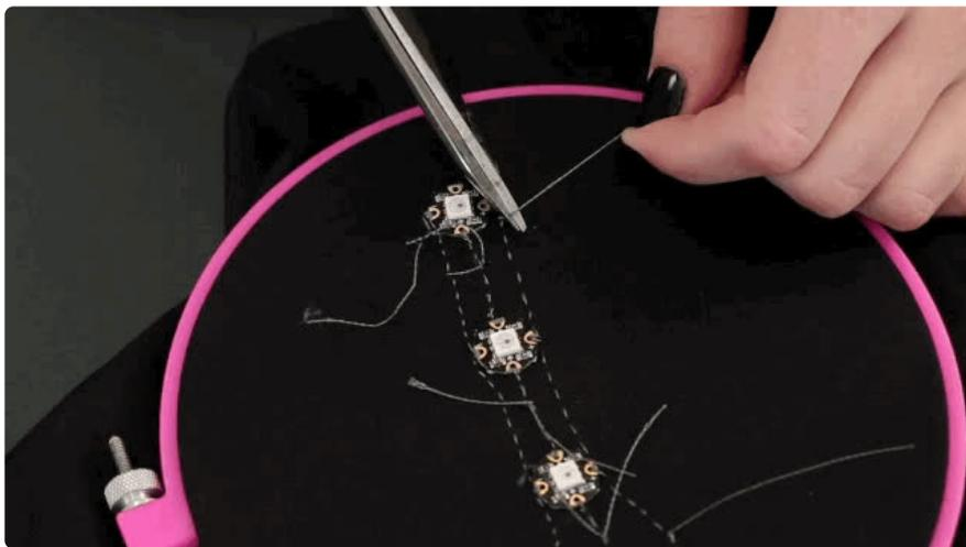
Double check your knots are secure before clipping all your thread tails. Clean up your work space so there aren't any stray bits of conductive thread hanging around.
