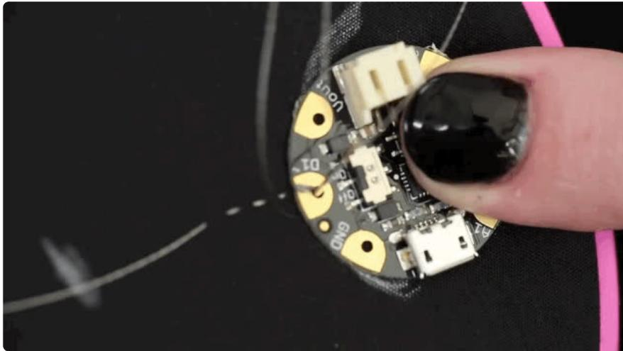
The pixels are chainable - so you only need 1 pin/wire to control as many LEDs as you like. They're easy to sew, and the chainable design means no crossed [conductive threads](http://adafru.it/641) (<http://adafru.it/641>). The output of one pixel connects directly to the input of the next.
