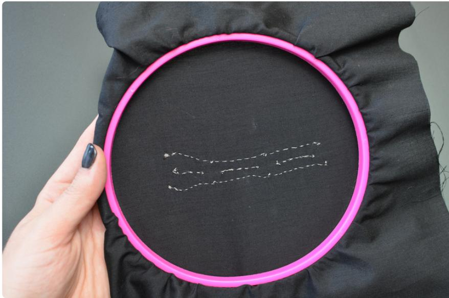
Here's what a three-pixel circuit looks like from the back. See the individual data connections in the center and the continuous power and ground buses above and below?
