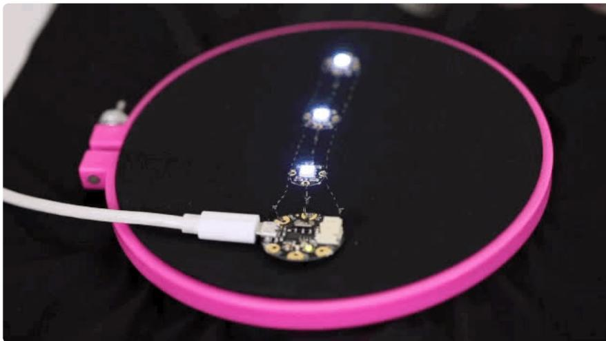
Plug your microcontroller into your computer with a USB cable. Change the number of pixels in the Arduino sketch or MakeCode project to match the number of pixels in your projects, and make sure the pin number matches what you sewed to. Upload the strandtest sample code as you did when testing a pixel earlier in this guide. Your pixels should light up and animate different colors and patterns.
