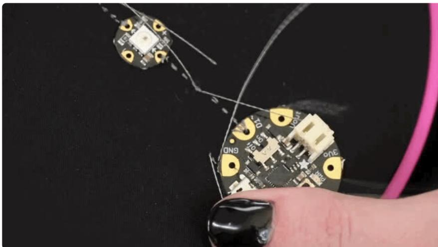
All the positive pads (marked with a +) connect together to form one power bus. Likewise all the negative pads (marked with a -) connect together to form one ground bus.
