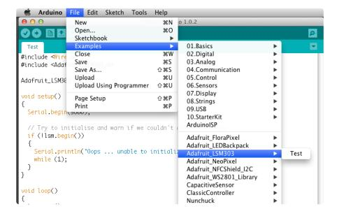
Open the special Adafruit version of the Arduino IDE and naviate to File-->Examples-->Adafruit\_LSM303--->Test to open the accelerometer test sketch. For more information on programming the Flora, check out the <u>Getting Started with FLORA</u> (https://adafru.it/aSZ) guide.
