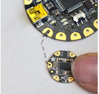
Stitch a path over to the gnd pad on the Flora accelerometer. When you get there, stitch a few times around the sensor's gnd pad.
