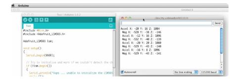
Open the serial monitor and watch the accelerometer values pour in!
