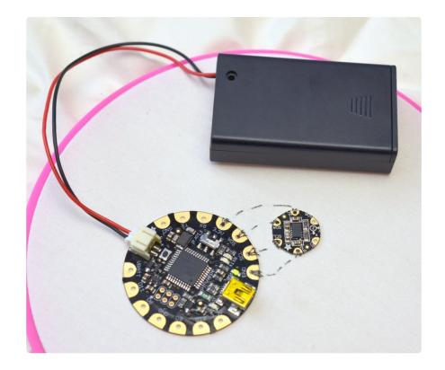
Modify this sample sketch to integrate this sensor into your project. Debugging over USB is helpful to see the ranges of numbers your sensor provides, but once your code is solid, you can disconnect from the computer and power your project with a 3xAAA battery holder.
