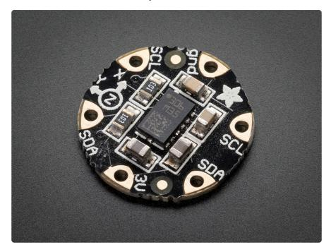
First let's get things moving. The <u>FLORA LSM303</u> (https://adafru.it/dN0) contains an accelerometer, which is great for detecting your dance moves, footsteps, or roller coaster rides. We've used it in the hem of the <u>Sparkle Skirt</u> (https://adafru.it/dN1) and on <u>3D printed wristband</u> (https://adafru.it/dN2) to flash some neopixels when you walk or shimmy.
