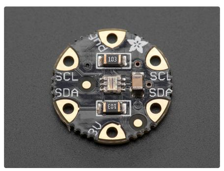
Now let's shed some light on the TSL2561 luminosity sensor. It'll read visible light, infrared, or both. Maybe you could make a darkness-activated headlamp or a hat that detects infrared security cameras.
