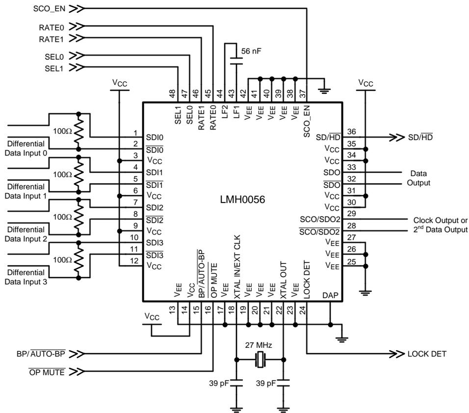
Figure 5. Application Circuit
