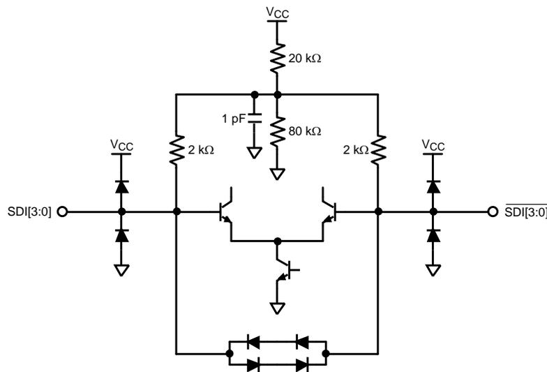
Figure 2. Equivalent SDI Input Circuit (SDI[3:0],  $\overline{\text{SDI[3:0]}}$ )
