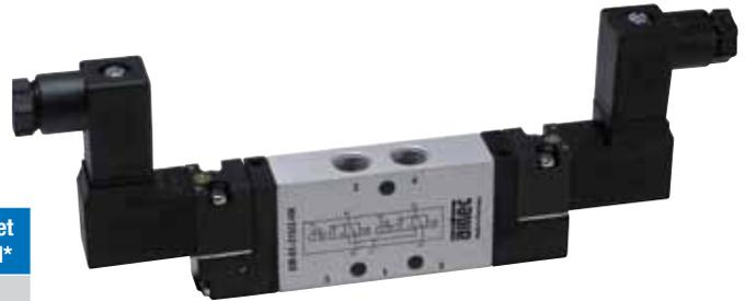
\* Manual override (HN) is on the side of ports 2 and 4 by default. It can easily be repositioned by 180° (side of ports 1, 3 and 5). When the valve is requested without the plug socket, the first digit of the order code for standard coils must be changed from 1 to 4. For optional plug sockets, see page 12.
