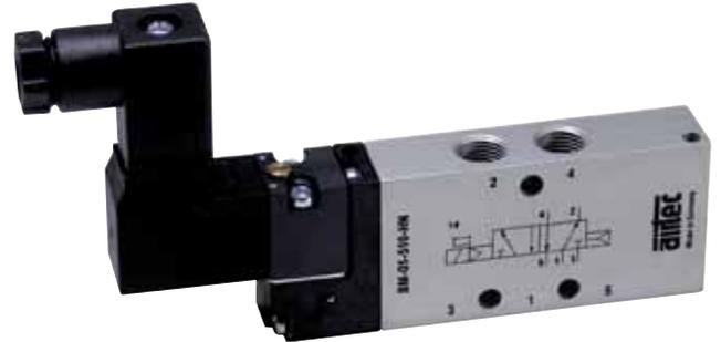
\* Manual override (HN) is on the side of ports 2 and 4 by default. It can easily be repositioned by 180° (side of ports 1, 3 and 5). When the valve is requested without the plug socket, the first digit of the order code for standard coils must be changed from 1 to 4. For optional plug sockets, see page 12.
