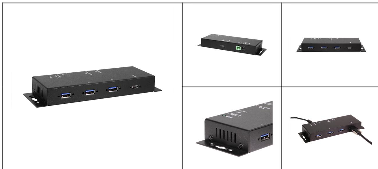
The CG-3X2C3AM is a USB3.1 Gen 1 Type-C PD (Power Delivery) Metal Hub that complies with the Universal Serial Bus (USB) Specifications Revision 3.1 Gen 1 and works up to 5Gbps. It provides 1 USB-C PD-Source capable upstream port and 4 downstream facing ports with 1 USB-C and 3 USB-A connectors.
