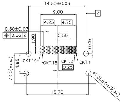
Recommended PCB Layout Connector Side
