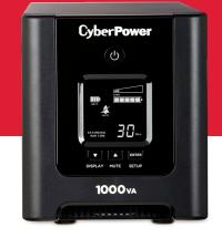
A mini-tower UPS with line interactive topology, the CyberPower PFC Sinewave OR1000PFCLCD provides power protection (using sine wave output) and surge protection for department servers, workgroup servers, network devices, telecom appliances, and high-end audio/video equipment requiring PFC power source compatibility.
