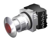
30mm Command/52, Chrome Finish Heavy Duty, Watertight/Oiltight Complete Metal Unit Illuminated Push-Pull Operator Transformer type, 120V AC LED Lamp Mushroom Head Cap Small 1 3/4" (44.5 mm) Metal, Chrome with Red Lens 2 Position Maintained, Pull-to-Release with 1 N.O. - 1 N.C. Heavy Duty Contacts, A600/P600 UL Listed, CSA Certified NEMA 1,3,3R,4,4X,12,13 & Automotive Standards
