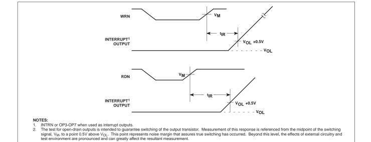
Figure 6. Interrupt Timing
