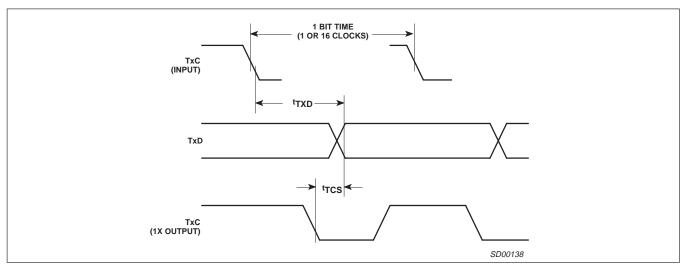
Figure 8. Transmitter External
