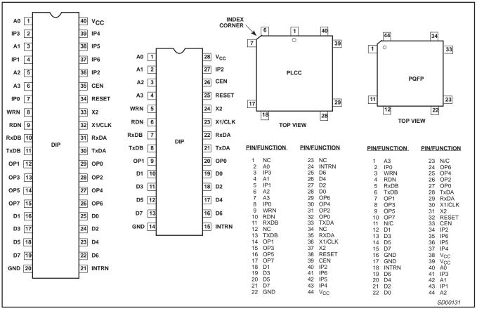
Figure 1. Pin Configurations
