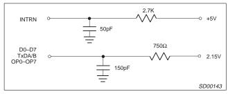
Figure 13. Test Conditions on Outputs
