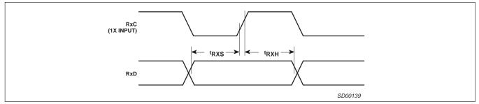
Figure 9. Receive External Clock
