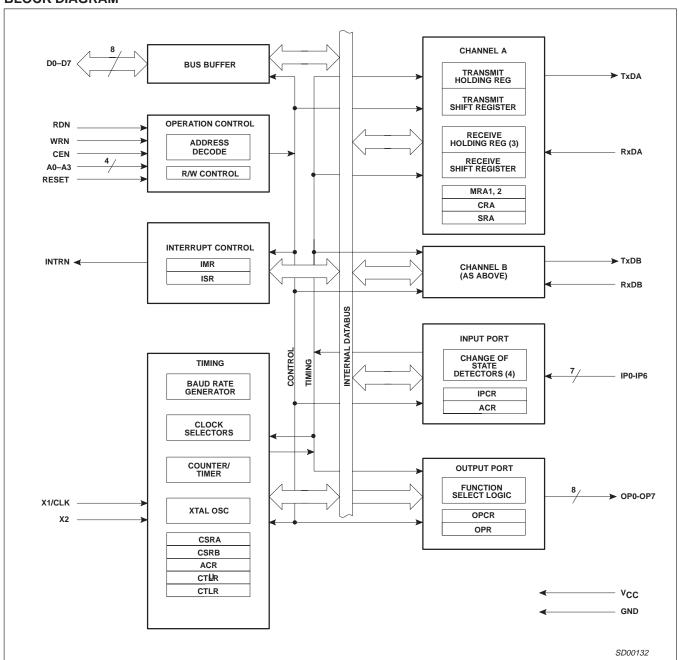
Figure 2. Block Diagram
