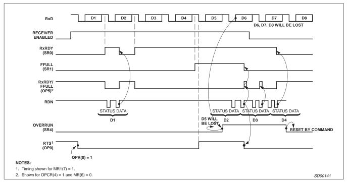
Figure 11. Receiver Timing
