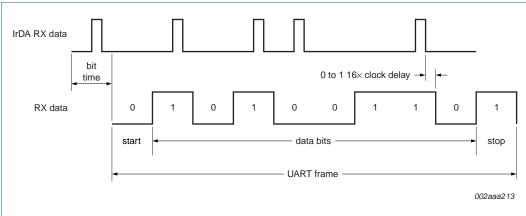
Fig 31. Infrared receive timing
