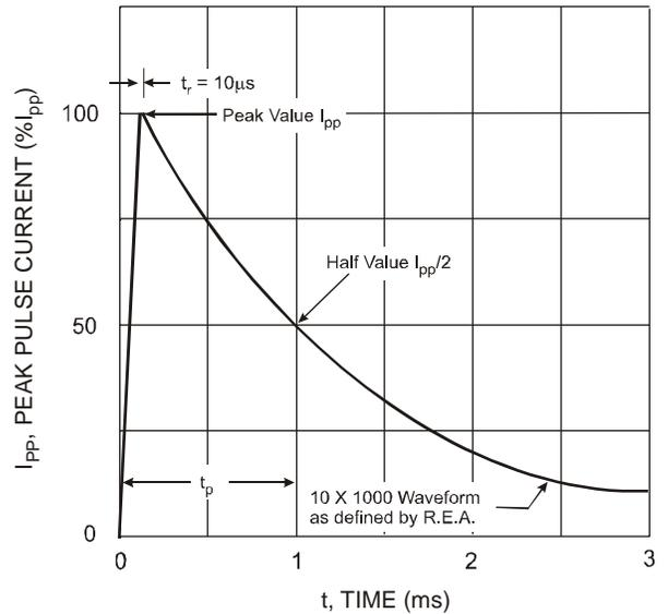
Figure 4. Pulse Waveform
