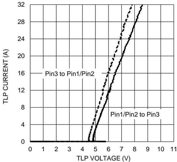
Figure 5 TLP Curve ( $t_p = 100\text{ns}$ )
