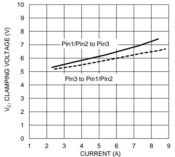
Figure 6 Clamping Voltage Characteristic ( $t_p = 8/20\mu\text{s}$ )
