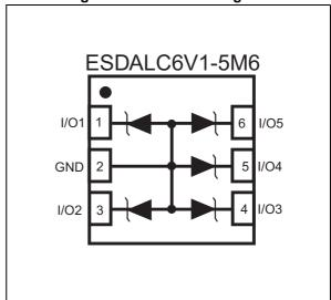
Figure 1. Functional diagram
