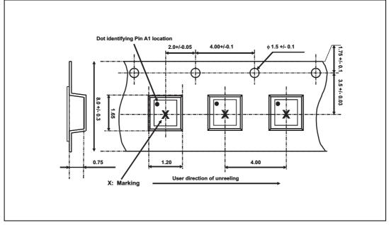
Figure 15. Tape and reel specification
