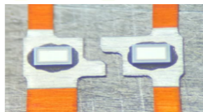
Die attach photo on new LF
