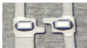
Die attach photo on old LF
