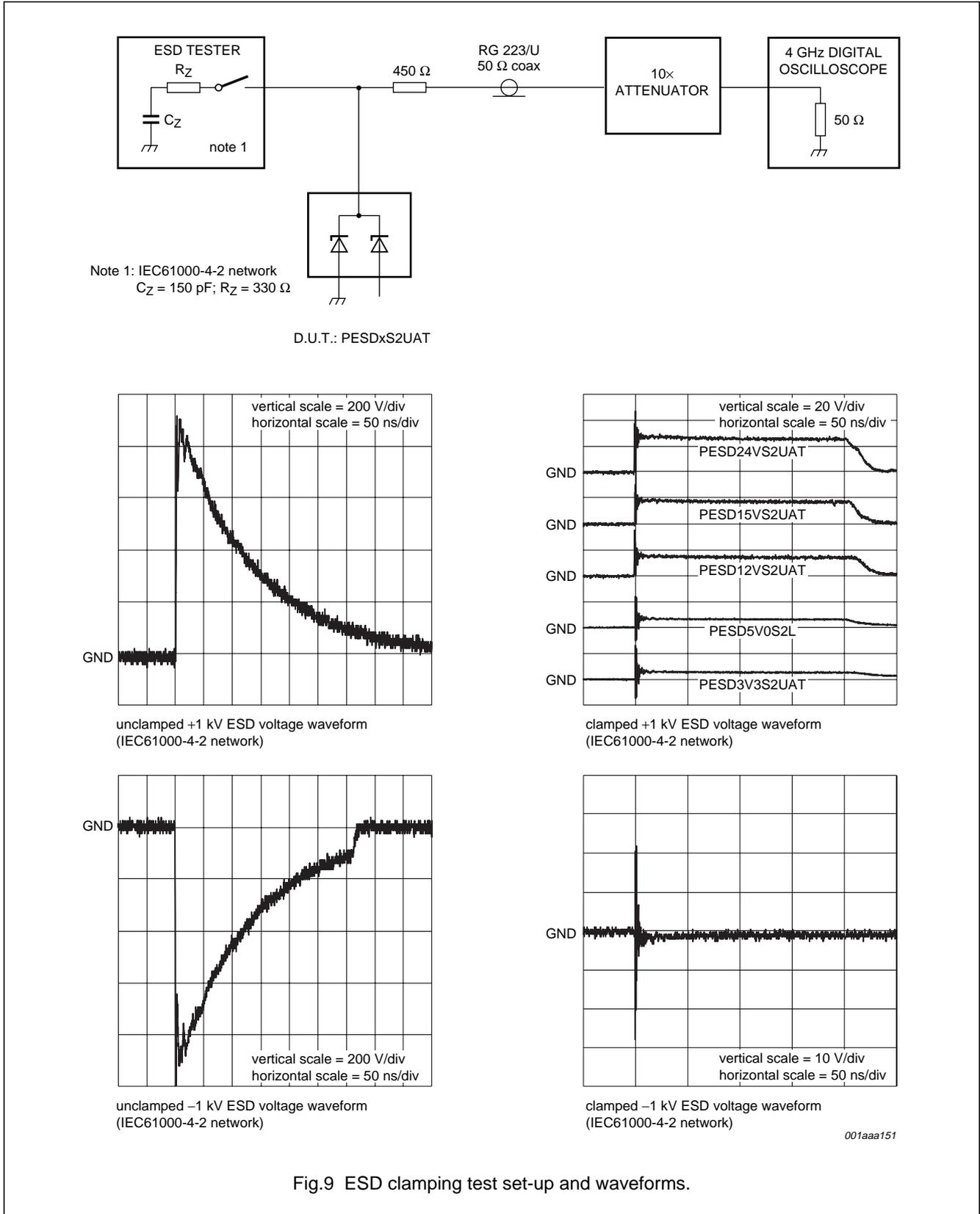
Fig.9 ESD clamping test set-up and waveforms.
