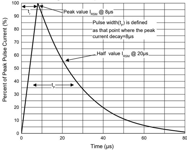
Fig. 2 - Non-Repetitive Peak Pulse Power
