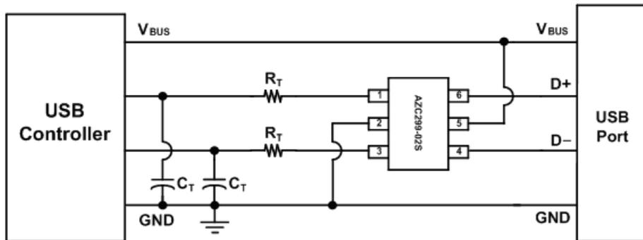
**Fig. 4 ESD Protection scheme for USB port by using AZC299-02S.**
