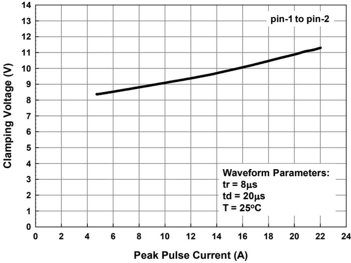
Forward Clamping Voltage vs. Peak Pulse Current
