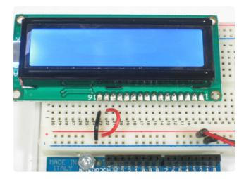
Connect the Arduino up to power, you'll notice the backlight lights up.
