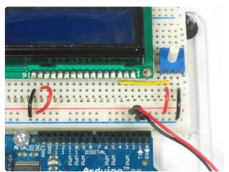
Connect one side of the pot to +5V and the other to Ground (it doesn't matter which goes on what side). The middle of the pot (wiper) connects to pin 3 of the LCD.
