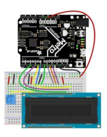
Board 5V to LCD pin 2, 15, and one side of the potentiometer. Board GND to LCD pin 1, 5, and the opposite side of the potentiometer. Potentiometer output (middle pin) to LCD pin 3 Board D7 to LCD pin 4 Board D8 to LCD pin 6 Board D9 to LCD pin 11 Board D10 to LCD pin 12 Board D11 to LCD pin 13 Board D12 to LCD pin 14 Board D3 to LCD pin 16 (red backlight) Board D5 to LCD pin 17 (green backlight) Board D6 to LCD pin 18 (blue backlight)
