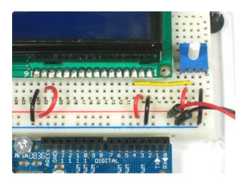
Now we'll wire up the logic of the LCD this is seperate from the backlight! Pin 1 is ground and pin 2 is +5V.
