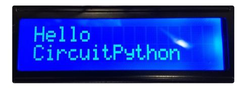
You can turn the cursor on and off using the **cursor** property. Set to True to turn it on and False to turn it off, for example to turn on:
