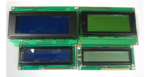
Although they display only text, they do come in many shapes: from top left we have a 20x4 with white text on blue background, a 16x4 with black text on green, 16x2 with white text on blue and a 16x1 with black text on gray.
