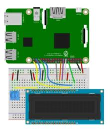
Pi 5V to LCD pin 2, 15, and one side of the potentiometer. Pi GND to LCD pin 1, 5, and the opposite side of the potentiometer. Potentiometer output (middle pin) to LCD pin 3 Pi GPIO26 to LCD pin 4 Pi GPIO25 to LCD pin 6 Pi GPIO25 to LCD pin 11 Pi GPIO25 to LCD pin 12 Pi GPIO22 to LCD pin 13 Pi GPIO27 to LCD pin 14 PI GPIO21 to LCD pin 16 (red backlight) Pi GPIO12 to LCD pin 17 (green backlight) Pi GPIO18 to LCD pin 18 (blue backlight)
