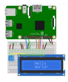
Pi 5V to LCD pin 2, 15, and one side of the potentiometer. Pi GND to LCD pin 1, 5, 16, and the opposite side of the potentiometer. Potentiometer output (middle pin) to LCD pin 3 Pi GPIO26 to LCD pin 4 Pi GPIO19 to LCD pin 6 Pi GPIO25 to LCD pin 11 Pi GPIO24 to LCD pin 12 Pi GPIO22 to LCD pin 13 Pi GPIO27 to LCD pin 14
