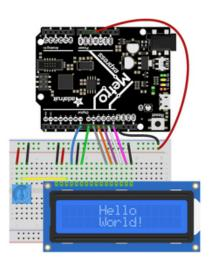
Board 5V to LCD pin 2 and one side of the potentiometer. Board GND to LCD pin 1, 5, 16, and the opposite side of the potentiometer. Potentiometer output (middle pin) to LCD pin 3 Board D7 to LCD pin 4 Board D8 to LCD pin 6 Board D9 to LCD pin 11 Board D10 to LCD pin 12 Board D11 to LCD pin 13 Board D12 to LCD pin 14 Board D13 to LCD pin 15 Remember just like the Arduino wiring page mentions there are 4 unused pins on the LCD, pins 7-10.
