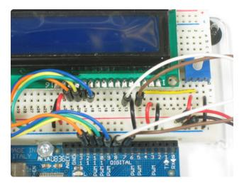
Next are the remaining 3 data lines, **DB6** (pin #13 yellow) **DB5** (pin #12 green) and **DB4** (pin #11 blue) which we connect to Arduino #**11**, **10** and **9**.
