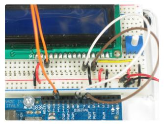
Now we will wire up the data pins. **DB7** is pin #14 on the LCD, and it connects with an orange wire to Arduino #**12**.
