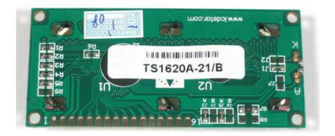
For this part of the tutorial, we'll be using LCDs with a single strip of 16 pins as shown above. There are also some with 2 lines of 8 pins like so:
