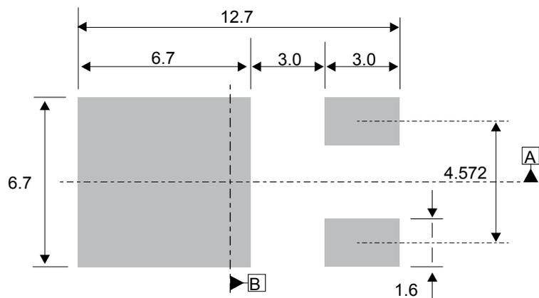
The device must be positioned within  $\oplus 0.05$  AB
