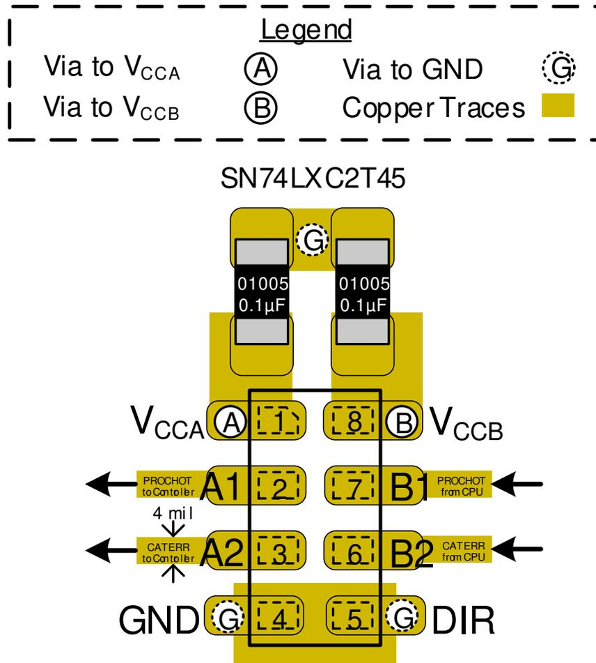
Figure 11-1. Layout Example—SN74LXC2T45DTT
