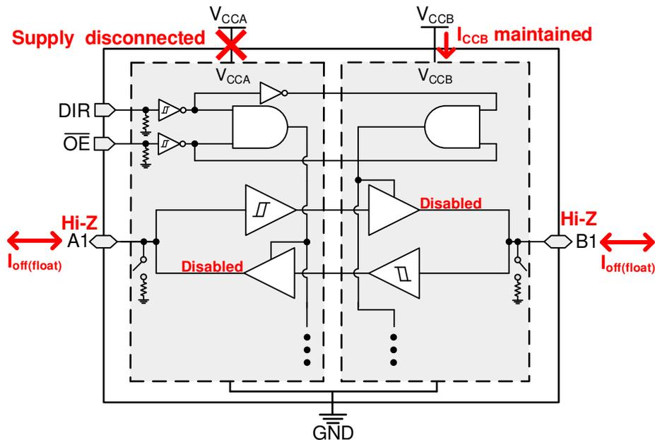
Figure 8-1. V<sub>CC</sub> Disconnect Feature
