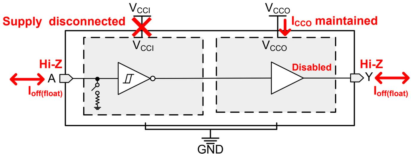
Figure 8-1. V<sub>CC</sub> Disconnect Feature
