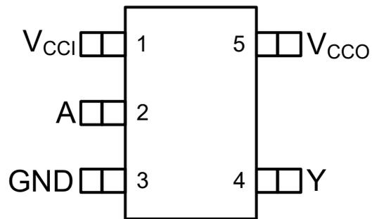
Figure 5-1. DCK Package, 5-Pin SC70 (Top View)
