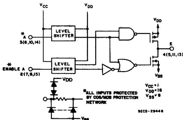
Fig. 1 – CD40109B logic diagram (1 of 4 units).
