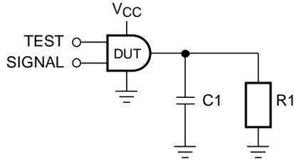
Figure 4. Test Circuit
