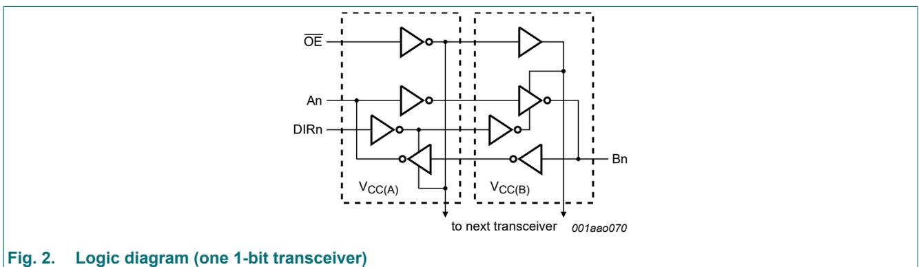
Fig. 2. Logic diagram (one 1-bit transceiver)
