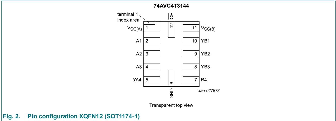
Fig. 2. Pin configuration XQFN12 (SOT1174-1)
