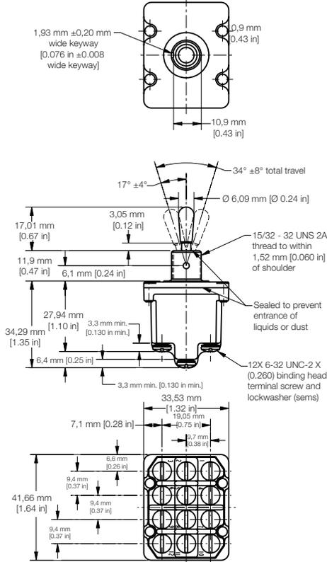
**14TL1: Four-pole, standard lever, solder terminals**
