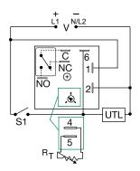
V = Voltage S1 = Initiate Switch C = Common, Transfer Contact NO = Normally Open NC = Normally Closed UTL = Untimed Load
