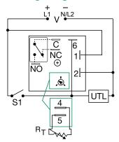
V = Voltage S1 = Initiate Switch C = Common, Transfer Contact NO = Normally Open NC = Normally Closed UTL = Untimed Load (optional)
