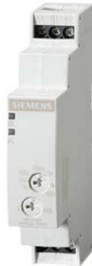
Timing relay, electronic OFF delay with control signal, 1 change-over contact 7 time ranges, 0.05 s...100 h 12-240 V AC/DC with LED, Screw terminal
