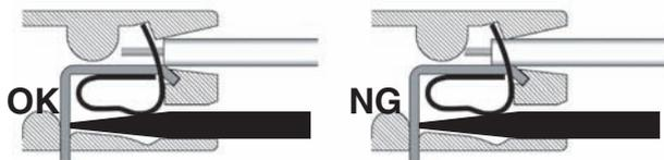
**2.** If the overall diameter of the wire is over 2.8 mm, it will be difficult to use double wiring.
