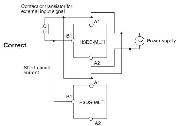
The H3DS Series is provided with a transformerless power supply system.
