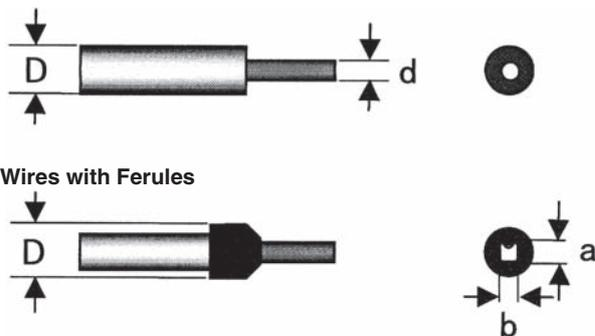
**Note: 1.** If the overall diameter of the wire is less than 1.8 mm, do not insert the wire past the conductor. Refer to the following diagrams.
