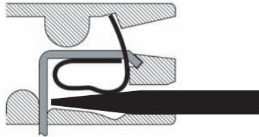
2. Insert the exposed conductor into the wire connection hole.
