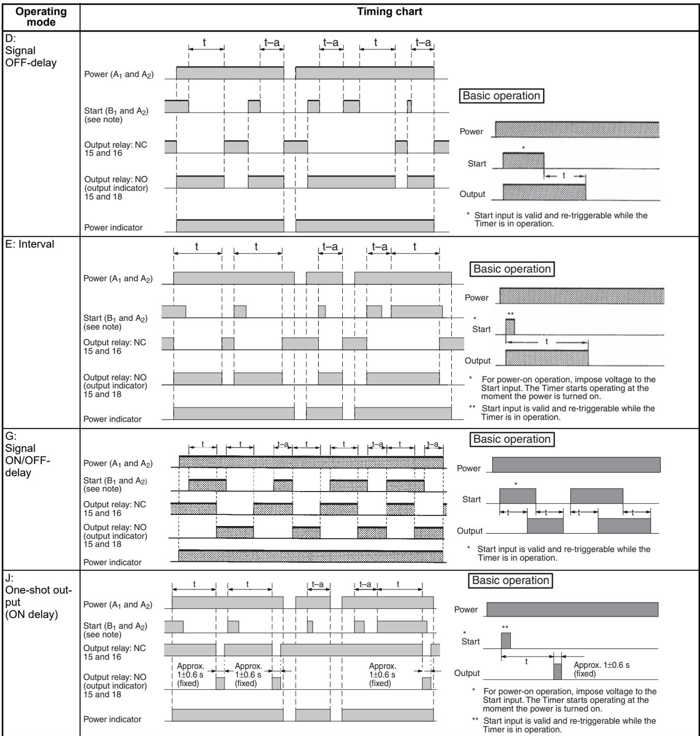
**Note:** The start input of the H3DS-ML□ model is activated by applying a voltage to B1 and A2 terminals.
