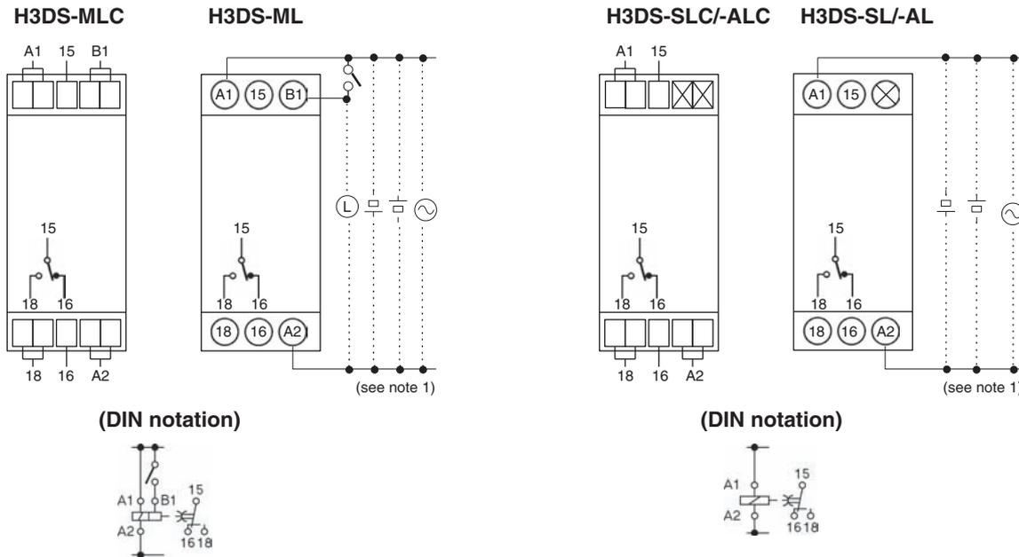
**Note: 1.** DC supply voltage does not require the designation of polarity.
