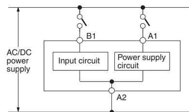
Since the input circuit and the power supply circuit are configured independently, the input circuit can be turned on or off irrespective of the on/off state of the power supply. It must be noted that a voltage equivalent to the power supply voltage is applied to the input circuit.
