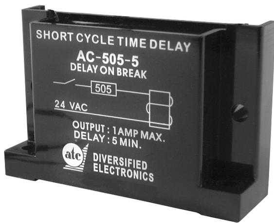
The **AC-505-5** provides **short cycle protection** by locking out the compressor for a period of time after a voltage or thermostat interruption. Subsequent interruptions will not increase the delay period. Since the delay begins when the interruption occurs, the temperature control is not affected. Under normal operating conditions, the compressor off time is longer than five (5) minutes. In this case, the use of these timers will not lengthen this off cycle.
