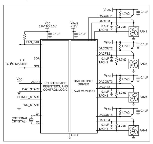
Figure 57. The MAX6620 shown here is a 4-channel linear fan speed controller using external pass transistors to supply variable power to the fans.
