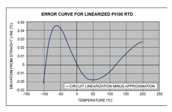
Figure 43. Error curve showing the deviation from linearity between -100°C and +200°C for the output of the circuit in Figure 42.
