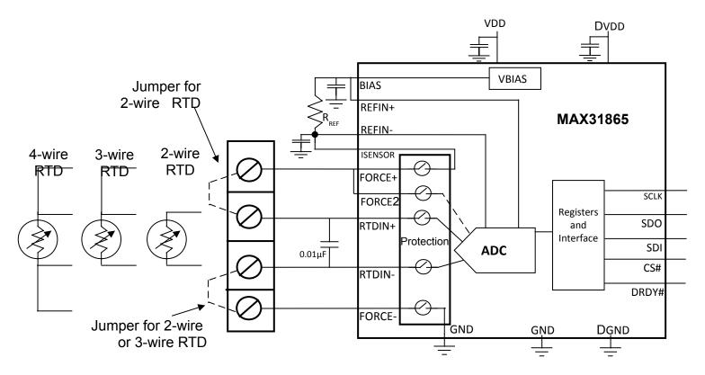
Figure 41c.2-, 3-, and 4-wire interface for PT100 or PT1000 RTDs using the MAX31865 RTD digitizer.
