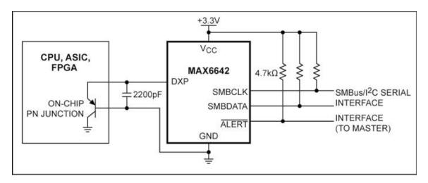
Figure 15. A remote temperature sensor monitoring the temperature of a sensing transistor (or thermal diode) on the die of an external IC.
