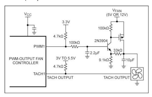
Figure 55. Circuit for converting PWM fan control signals to a linear supply voltage.
