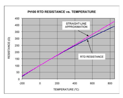
Figure 4. PT100 RTD resistance vs. temperature. Also shown is the straight-line approximation for 0°C to +100°C.
