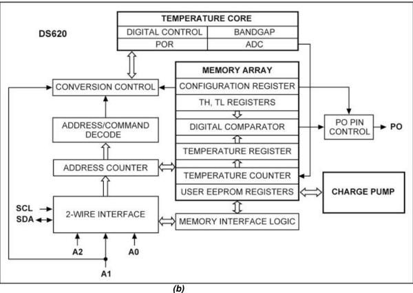
Figure 14. Block diagrams of local digital temperature sensors. (a) Simple sensor with serial digital output. (b) Sensor with additional functions, such as over-/undertemperature alarm outputs and user EEPROM.
