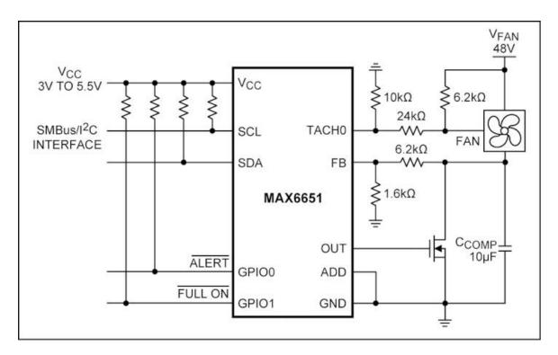
Figure 60. 48V, linear fan RPM controller. The feedback and tachometer signals are attenuated for compatibility with the MAX6651's input voltage tolerance.
