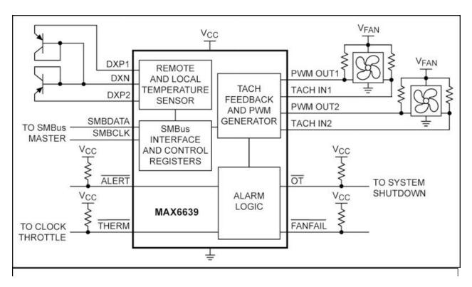
Figure 54. The MAX6639 controlling two 4-wire fans; it measures two temperatures and can control fan RPM based on the measured temperature.
