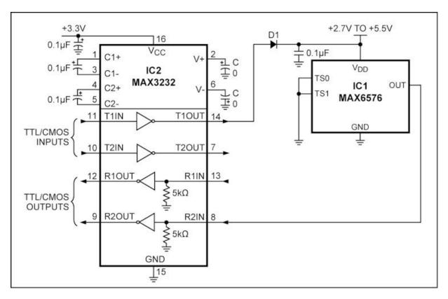
Figure 47. RS-232-powered temperature sensor.
