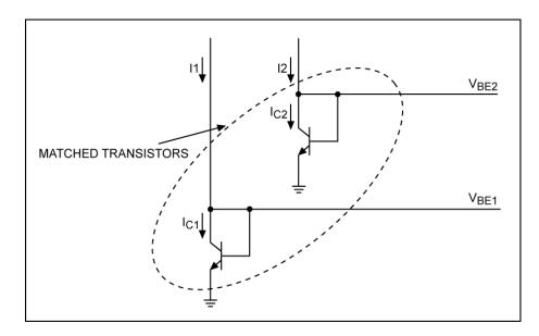
Figure 11. Conceptual circuit showing how two matched transistors can sense temperature.
