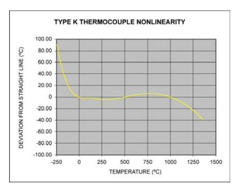
Figure 8. Type K thermocouple deviation from a straight-line approximation.
