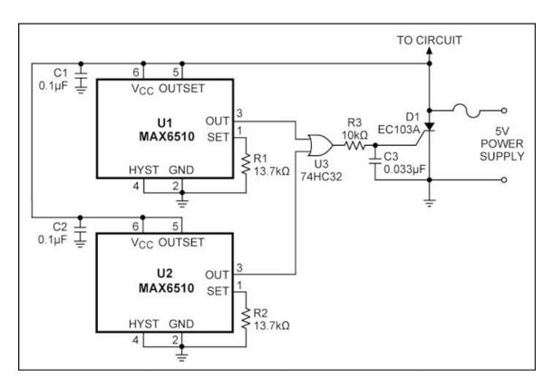
Figure 67. Overtemperature crowbar circuit with two temperature switches. If either temperature switch is hot enough to trip, SCR D1 will turn on, thus shorting the power supply and blowing the fuse.
