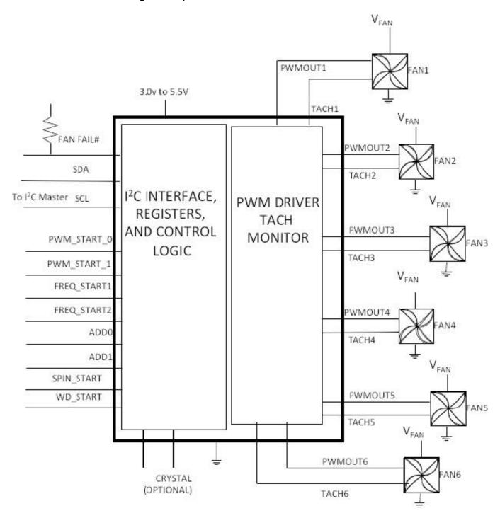
Figure 50. If the system microcontroller is capable of monitoring temperature sensors and determining the desired fan speeds, it can communicate the desired speeds to a fan speed
