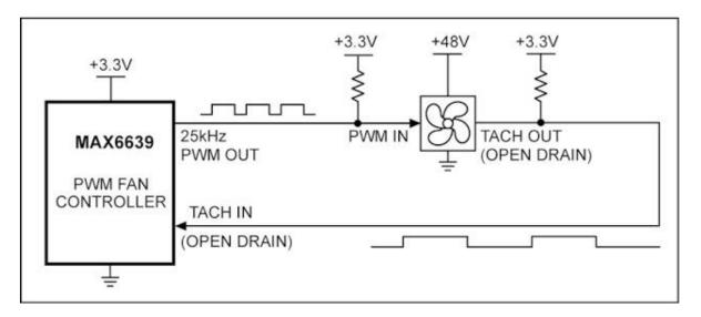
Figure 58. Controlling a 48V 4-wire fan. No special precautions are needed—any PWM-output fan controller with an appropriate output frequency available will work.
