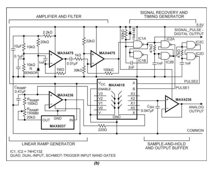
Figure 46. IR-linked temperature sensor. (a) Sensor and transmitter. (b) Receiver.
