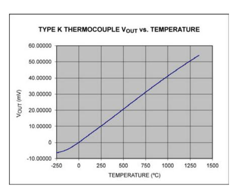
Figure 7. Type K thermocouple output voltage vs. temperature.
