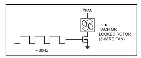
Figure 25. Controlling the speed of a 2- or 3-wire fan by pulse-width modulating the power supply using an n-channel FET on the low side of the fan.
