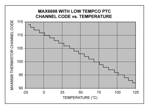
Figure 38. MAX6698 thermistor channel code vs. temperature when used with a 0.3%/°C integrated thermistor.
