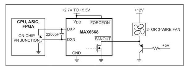
Figure 64. Remote, two-speed fan controller with factory-set threshold. Below the threshold, the fan runs at approximately half speed. Above the threshold, it runs at full speed.
