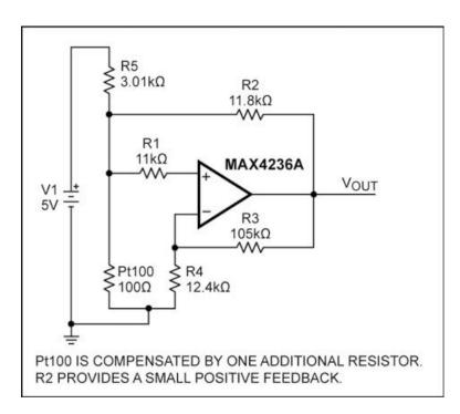
Figure 42. PT100 linearizer circuit.
