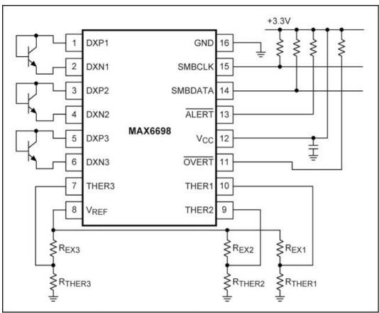
Figure 30. The MAX6698 includes a local temperature sensor, inputs for three external sensing transistors, and inputs for three NTC thermistors ( $R_{THER3}$ ).
