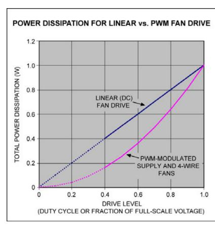
Figure 24. Comparison of power dissipation in linear (upper curve) and PWM fan drive (lower curve) approaches.
