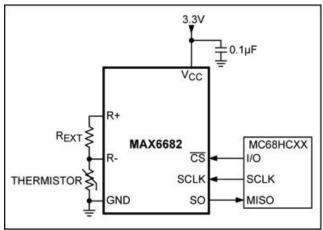
Figure 31. MAX6682 single thermistor-to-digital converter.
