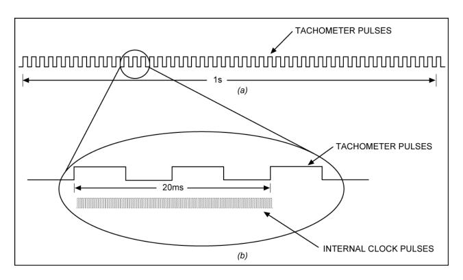
Figure 26. (a) Monitoring fan speed by counting tachometer pulses for a period of 1s can result in low-resolution measurements. (b) Generating a clock signal with sufficiently high frequency, and then counting the number of clock pulses in a limited number of tachometer periods, provides more resolution and allows the fan's RPM to be controlled to within a tighter tolerance.
