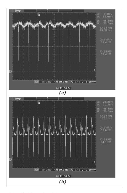
Figure 27. Examples of fan supply current waveforms. (a) A fan driven with half the nominal power supply voltage. (b) The same fan driven with the nominal power supply voltage.
