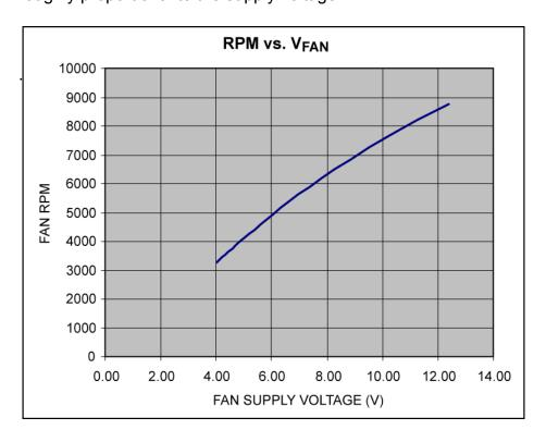
Figure 22. Fan RPM vs. power supply voltage for a typical 12V fan.
