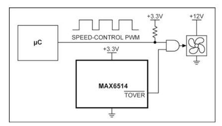
Figure 65. Fan fail-safe circuit with factory-set trip threshold
