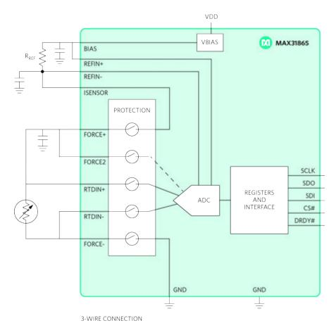
Figure 32.The MAX31865 digitizes the resistance of a 2-, 3-, or 4-wire RTD, detects cable and sensor faults, and includes ±45V input protection.
