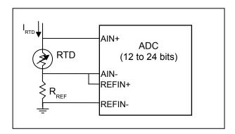
Figure 6. Simplified RTD signal-conditioning circuit.
