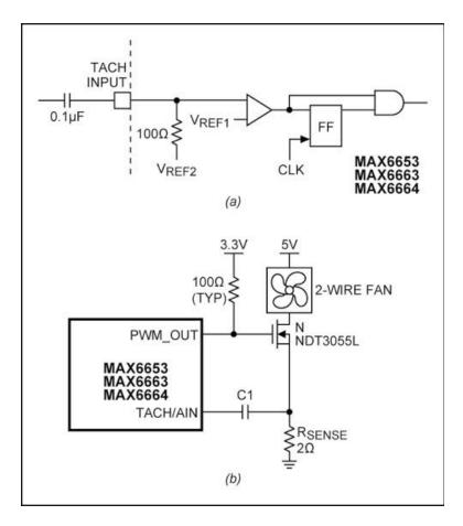
Figure 28. (a) Typical input stage for monitoring fan speed using the fan's supply current. (b) Using this input stage to monitor fan speed using a  $2\Omega$  sensing resistor.
