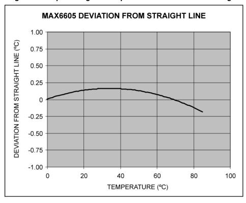
Figure 13. The MAX6605 output voltage deviation from a straight line. Linearity from 0 °C to +85 °C is approximately  $\pm 0.2$  °C.
