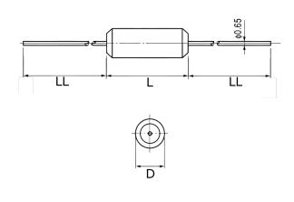
**General Information** Series TRS Thermal Reed Switch Type Style Axial Description Thermal Reed Switch High Reliability, High-Speed Response, Long Features Operational Life, Excellent Environmental Durability, High Temperature Accuracy Lead Wire Leads RoHS Yes REACH Yes
