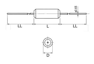
**General Information** Series TRS Thermal Reed Switch Туре Style Axial Description Thermal Reed Switch High Reliability, High-Speed Response, Long Features Operational Life, Excellent Environmental Durability, High Temperature Accuracy Lead Wire Leads RoHS Yes REACH Yes
