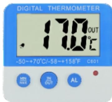
2. When the 1st setup temperature HIGHER than the 2nd setup temperature, the current alarm range is over 1st setup temperature or below 2nd setup temperature.
