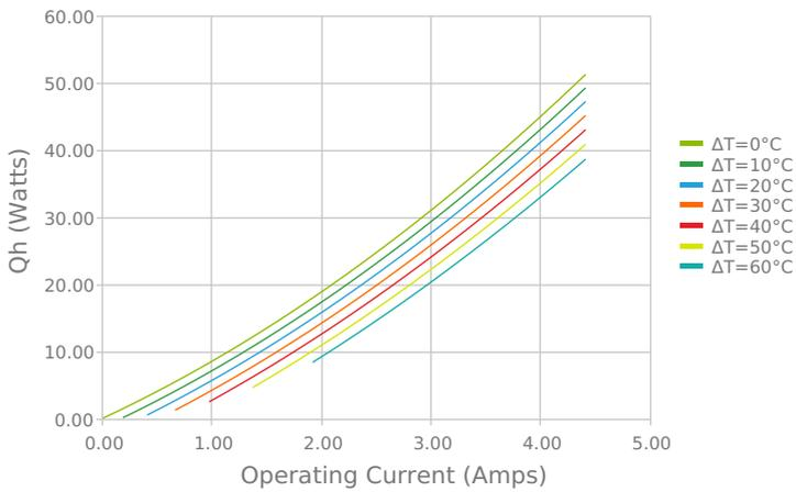
Total Heat Dissipated at Hot Side (Qh=Qc+Pin)
