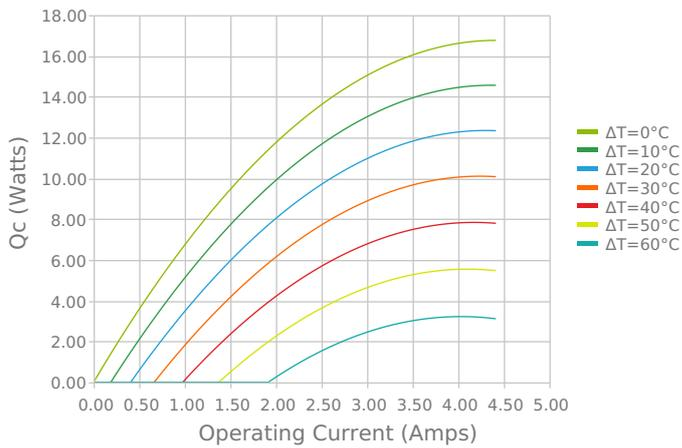
Heat Pumped at Cold Side
