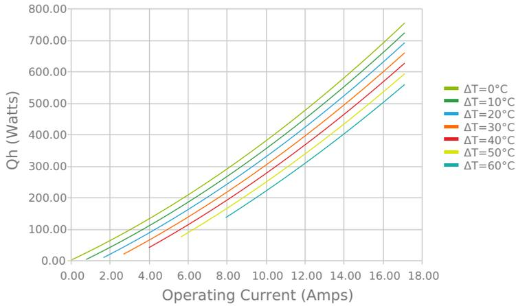
Total Heat Dissipated at Hot Side (Qh=Qc+Pin)
