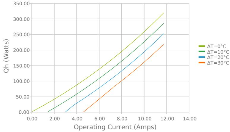
Total Heat Dissipated at Hot Side (Qh=Qc+Pin)
