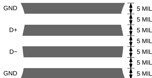
Figure 34. Typical Arrangement of Signal Tracks
