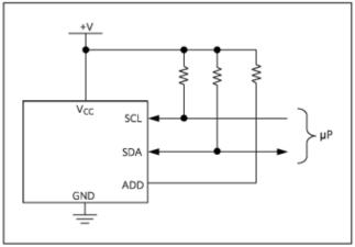
Figure 1. Input-level-defined addressing as implemented in the DS1621, DS75, or MAX6634 temp sensors. When this function is used, then multiple temperature devices like these can have their own slave address.
