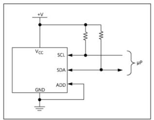
Figure 2. Pin-state-defined addressing, as implemented in the MAX6650 or MAX6681 temperature sensors, allows for definition of the address pin with local, direct connections.
