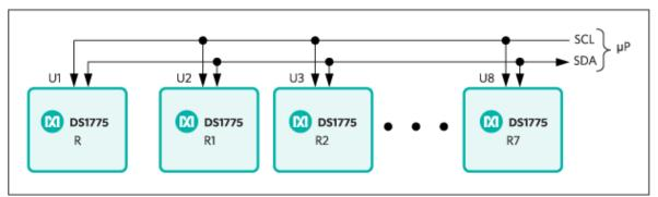
**Figure 4** depicts a simplified connection scheme utilizing eight unique DS1775 digital thermometer ordering variants.
