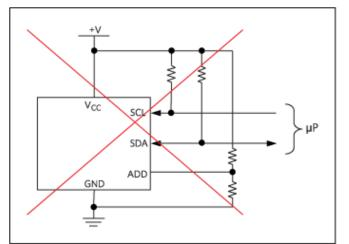
Figure 3. Do not use pullup or pulldown resistors on a "No Connection" pin configuration.
