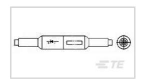
Terminal Junction System Component Type: Electronic Splice-Diode
