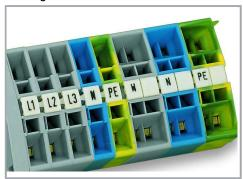
Marking via Mini-WSB Quick Marking System.
