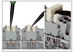
Removing a push-in type jumper bar: Insert the operating tool between the jumper and partition wall of the dual jumper slots, then lift up the jumper.
