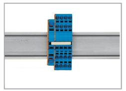
Stepping down via push-in type jumper bar: Commoning via closed terminal side with end plate allows jumpering over two cross-section sizes, e.g., from 16 mm² (6 AWG) to 6 mm² (10 AWG) or from 6 mm² (10 AWG) to 2.5 mm² (14 AWG) (see illustration above).
